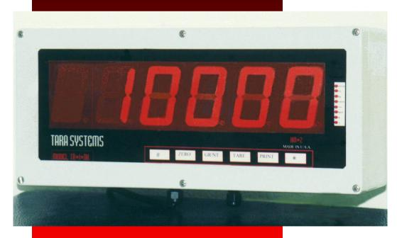
NTEP Legal for trade Industrial sealed polycarbonate enclosure 14 By 6 By 4 " All pushbutton controls Auto tare Lb to Kg conversion Printer output Computer output Super bright 2.2 high LED display Sealed operational buttons. Other type enclosures are available (stainless / steel) 12volt DC models available Made in U.S.A.
